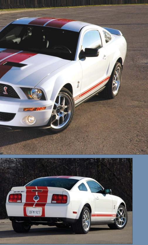
Ford's SVT engineers retuned and upgraded key Mustang chassis components. Improvements include revised shocks, spring rates and upgraded stabilizer bars. The basic GT500's unique design features include wide upper and lower fascia openings with a functional air splitter. On either side, slanting headlamp openings add to the dramatic front
