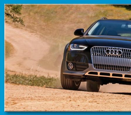
Safety and convenience electronics are plentiful, including adaptive front lights, Audi side assist (radarbased blind spot monitoring), and an optional driver assistance package, with adaptive cruise control, active lane assist and speed-sensitive steering. Active lane assist invokes steering correction if you start to wander outside your lane markings without having signaled.
