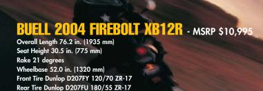
ENGINE: 1203cc air/oil/fan-cooled, four-stroke, 45 degree V-Twin Valve Train OHV, two valves per cylinder, self adjusting Fuel Delivery 49 mm downdraft DDFI II fuel injection Torque (North America Per SAE J607) 84 ft-lbs @ 6000 rpm Horsepower (North America Per SAE J607) 103 HP @ 6800 rpm
