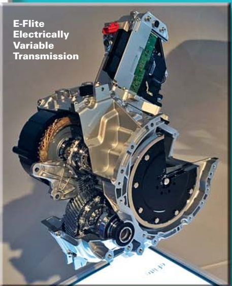
A core component of the Chrysler Pacifica Hybrid's eHybrid system is its E-Flite Electrically Variable Transmission (above), an in-house development which operates in both electric vehicle (EV) or hybrid electric vehicle (HEV) modes, utilizing two electric machines and planetary gear set with one-way clutch. The innovative one-way clutch enables both electric machines to drive the front wheels in electric-only mode.
