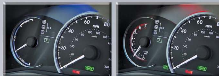
The CT 200h's size and weight are helped by an optimized hybrid powerplant and a compact NiMh battery pack. Contextual gauges show charging info with a blue glow in ECO mode, a tachometer and red glow in Sport.
