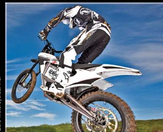
All the Zero electric bikes are mono-shock with chain drive. An exhaust tube is for an electric motor cooling fan.
